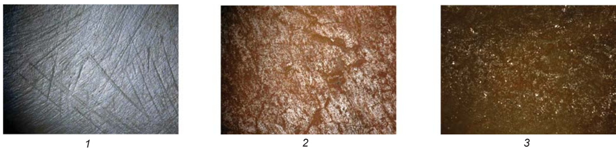
Fig. 6. Traces resulting from abrasive grinding of the working-area and from polishing the surface of pottery (1), from polishing a stone-axe (2) and a bronze article (3). 50x magnification. Experimental specimens. Quartz.
